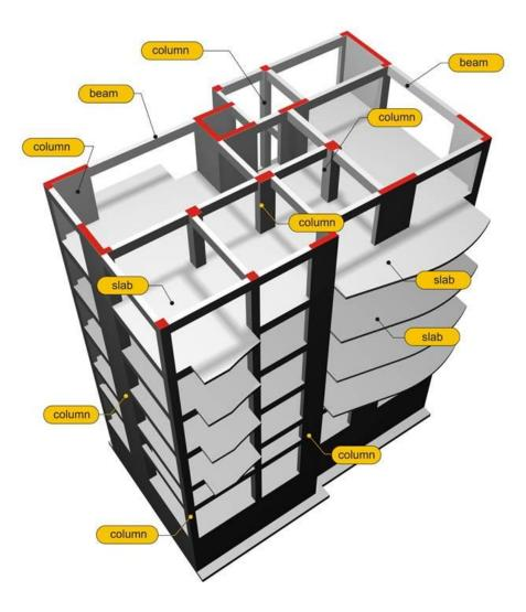
Figure 1: Super structural elements
