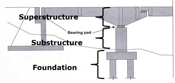
Fig. 7: Different parts of a Bridge
