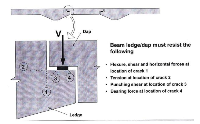
Fig.51 : Cracks at articulation
