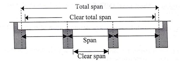
Fig. 12: Total span, total clear span, span and clear span
