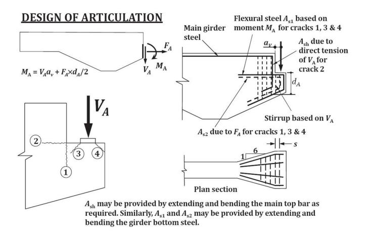
Flexural steel  $A_{s1}$  based on Main girder moment  $M_A$  for cracks 1, 3 & 4 Steel  $a_{V}$   $a_{sh}$  due to  $d_{irect}$  tension of  $V_A$  for crack 2  $a_{s1} =$   $a_{s2} =$   $a_{s2} =$   $a_{s2} =$   $a_{s2} =$  $a_{s2} =$
