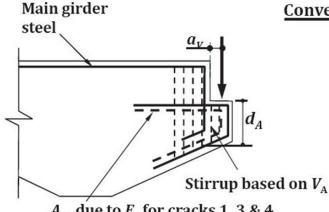
$A_{s2}$  due to  $F_A$  for cracks 1, 3 & 4 and  $A_{vf}$  from shear friction criterion
