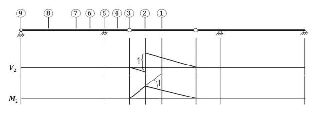
Fig. 39: IL diagram for shear and moment at section 2
