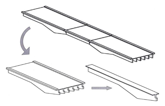
Fig.49 : Articulation or halving joint
