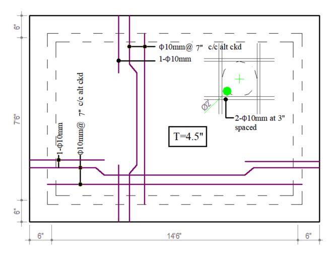
Figure 9: Reinforcement details of top slab overhead water reservoir
