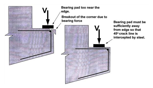
Fig.52 : Clearance requirement around bearing pad near articulation
