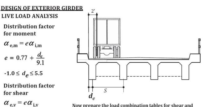
Now prepare the load combination tables for shear and moment. Dead load values shall be recalculated based on revised loading (DC and DW). Live load values may be directly copied from previous load combination tables and combinations may be performed with  $\alpha$  values for exterior girder.
