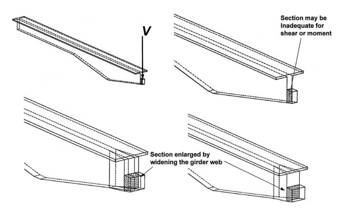
Fig.50: Widening of girder near articulation location
