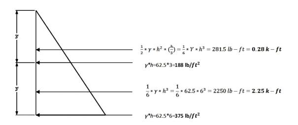
Figure 8: Pressure distribution on reservoir wall
