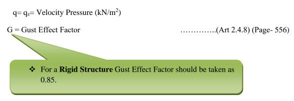
A building or other structure whose fundamental frequency  $(F = \frac{1}{T})$  is greater than or equal to 1 Hz then this building is known as Rigid Structure.
