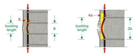
Figure 21: Failure mechanism of a column
