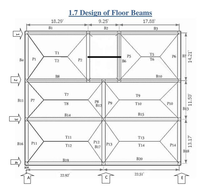
Figure 16: Beam layout
