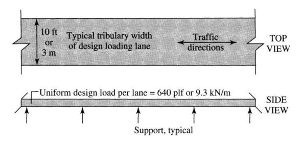
LANE load is NOT subjected to dynamic allowance (impact) Fig.27: Design Lane load
