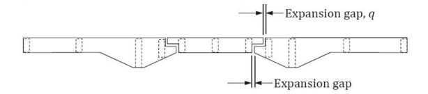
Expansion gap is required to accommodate the thermal expansion-contraction. In Bangladesh seasonal temperature varies between 5 °C to 40 °C. For the purpose of design we take  $\Delta t = 40$  °C.
