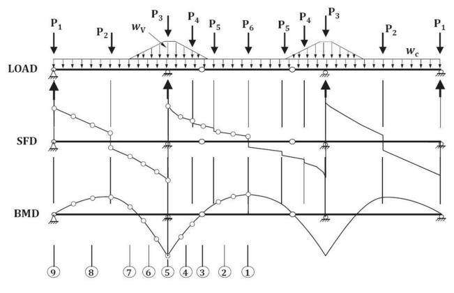
Fig. 37: SFD and BMD of interior girder due to DC dead load
