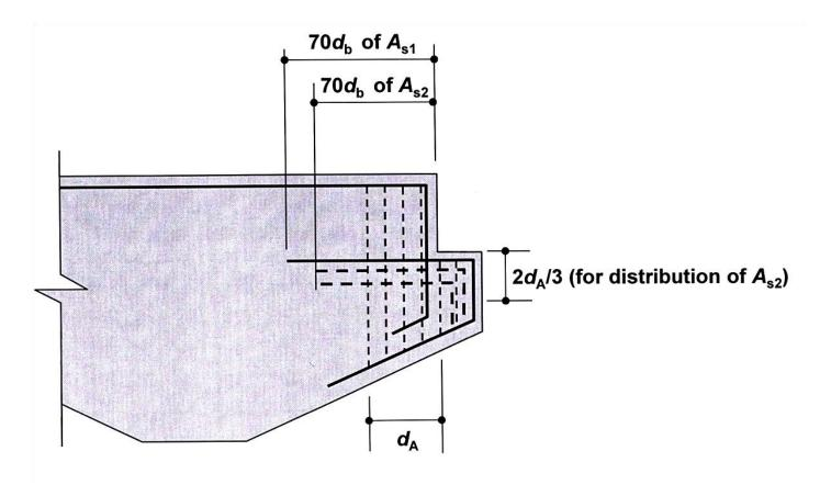
Fig.54 : Reinforcement detailing of articulation
