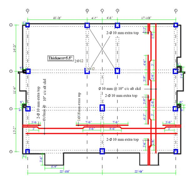
Figure 15: Typical Reinforcement Details of Slab
