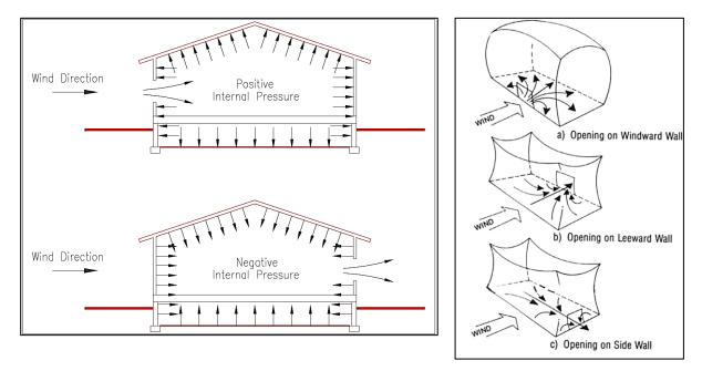
Figure: Internal Pressure
