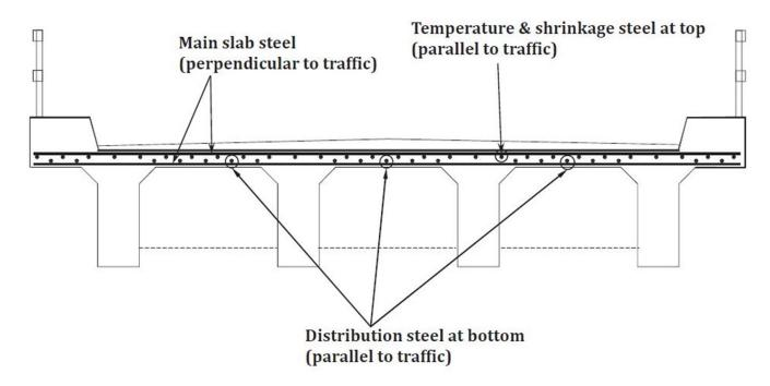
Fig.32: Reinforcement detailing of Slab
