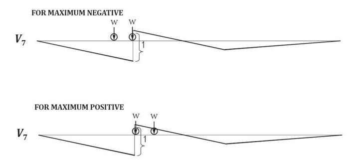
Fig. 43: Maximum positive & negative moment, shear at section 7 for tandem load
