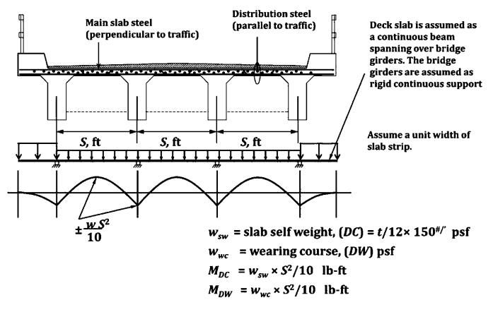
Fig. 30: Dead load on deck slab
