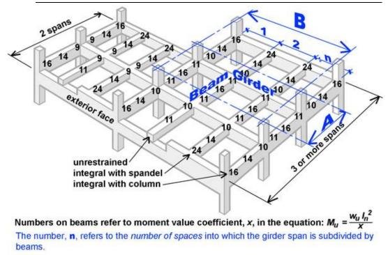
Figure 4: Moment coefficients for beam.
