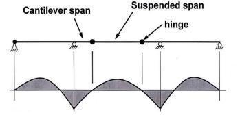
Fig. 15: A bridge having intermediate hinges
