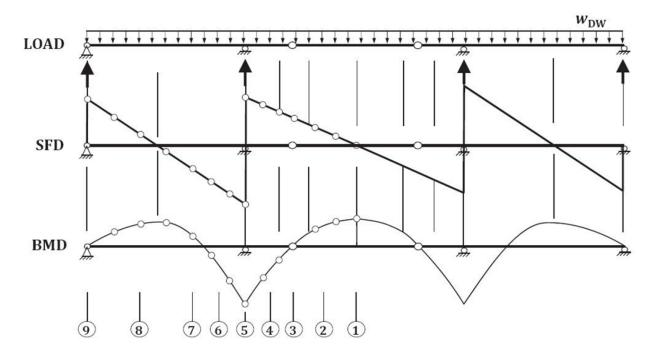
Fig. 38: SFD and BMD of interior girder due to DW dead load (wearing course)
