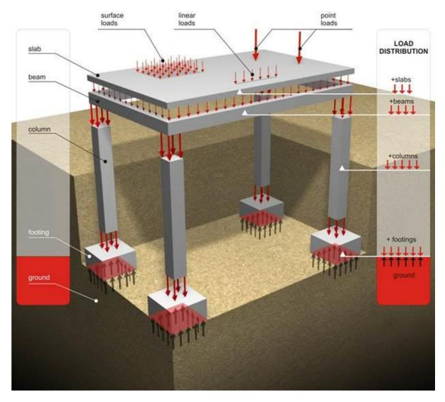
Figure 3: Gravity load distribution
