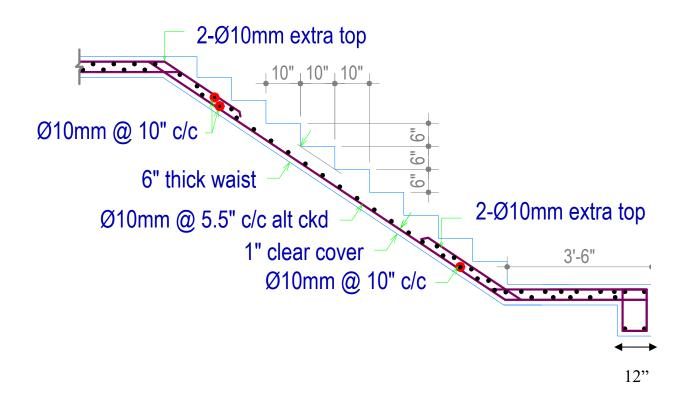
Figure 6: Reinforcement details of stair
