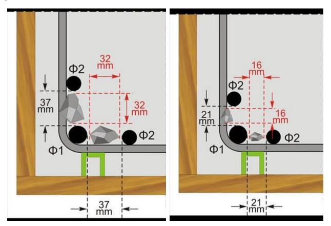
Figure 20: Minimum spacing between reinforcement bars
