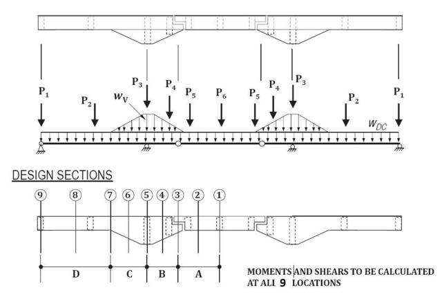
Fig. 36: Design sections of Interior Girder
