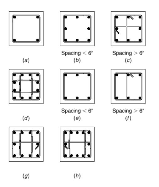
**Figure 22:** Tie arrangement of rectangular column ((Ref: ACI Code, Design of Concrete Structure, 13<sup>th</sup> edition, Chap-8, P-254)
