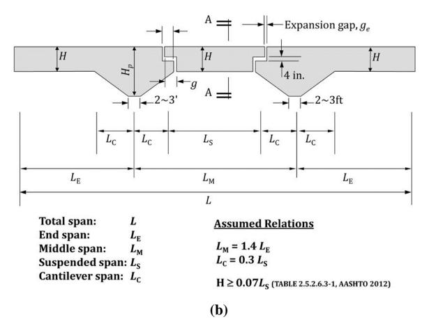
Fig.28: Longitudinal profile a three spanned balanced cantilever bridge
