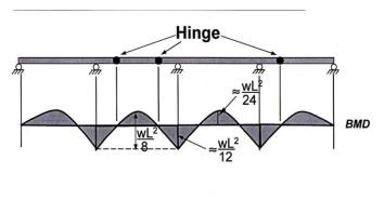
Hinges render the structure determinate:
