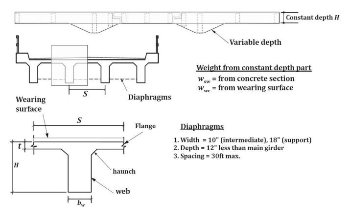
Fig. 35: Different dimensions of longitudinal girder
