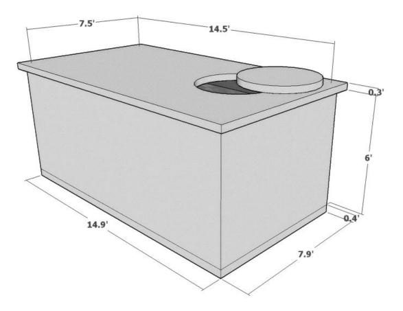
Figure 7: Roof top water reservoir (Overhead water reservoir)
