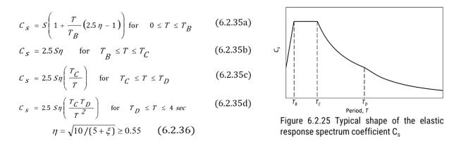
$\eta$  = Damping correction factor as a function of damping with a reference value of  $\eta$  = 1 for 5% viscous damping
