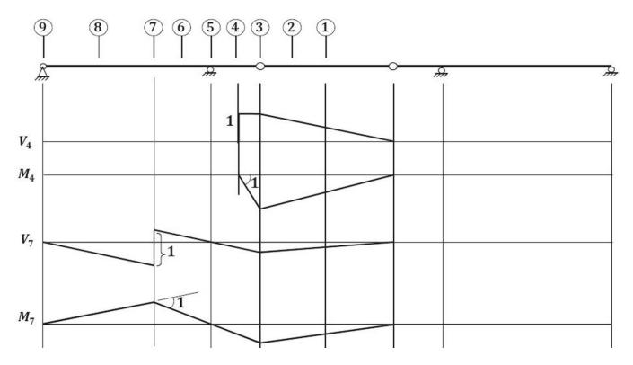
Fig. 40: IL diagram for shear and moment at section 4 and 7
