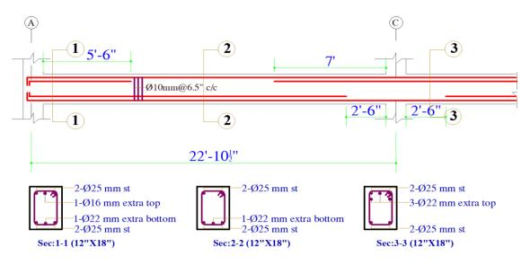
Figure 17: Reinforcement detail of beam
