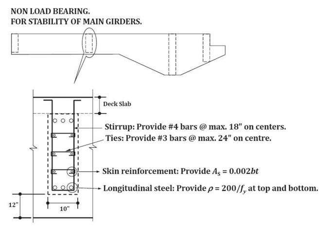
Fig.48 : Reinforcement detailing of cross girder
