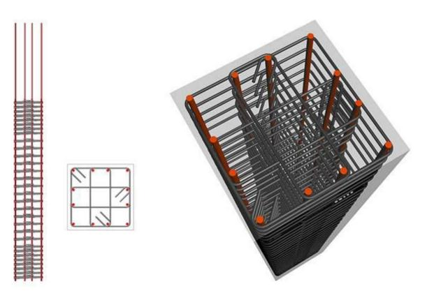
Figure 24: Typical column detail
